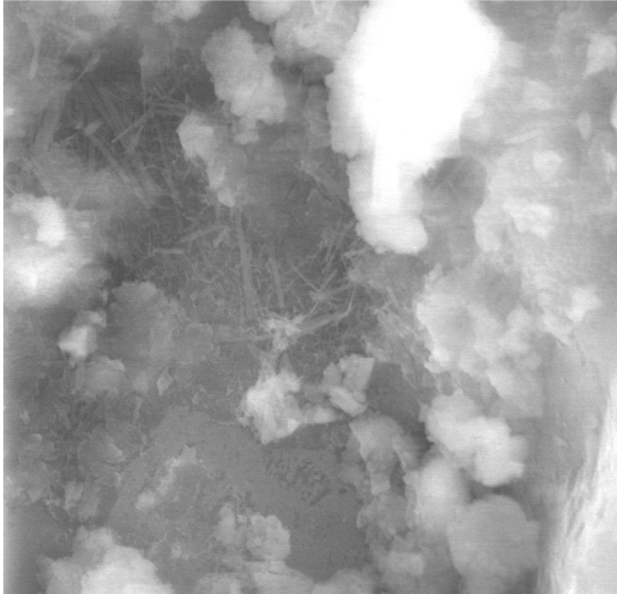
Fig.-5a: SEM image of Control mortar (28 Days)
