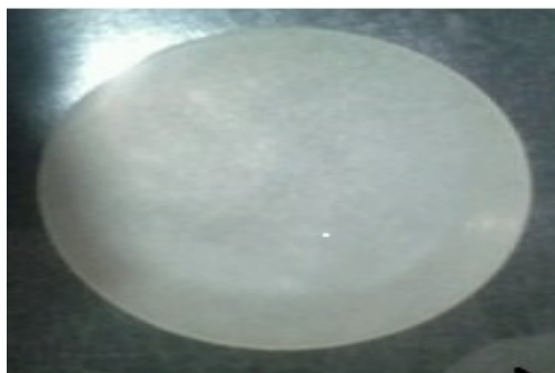
Fig.-1: PAN Complexed Gel polymer Electrolyte film with NaF salt
