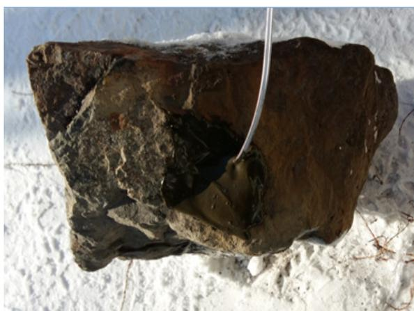
Fig.-2: A stone charged with a gas-generator charge
