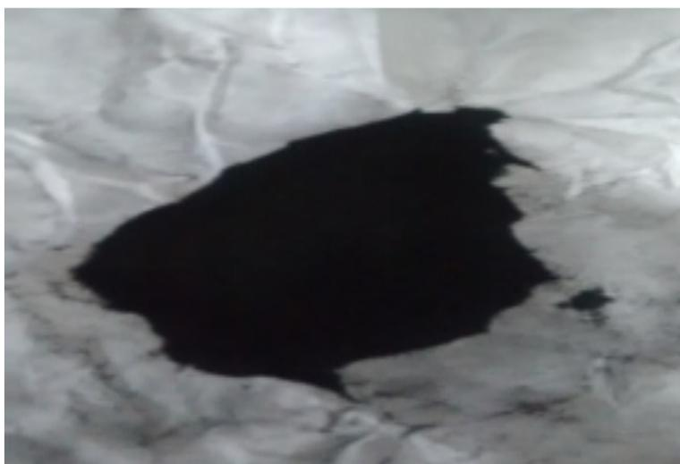
Fig.-3: Activated carbon from waste rubber tire
