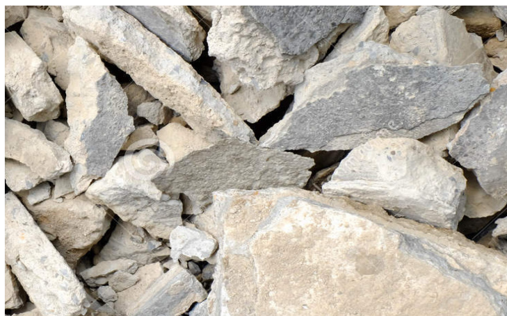
Fig.-6: Destruction of concrete gas generator chemical cartridge composition: oxidizer ( \text{NH}_4\text{NO}_3 ) - 60%; CNM - 20%; magnesium - 10%; smokeless powder - 10%
