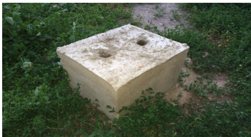
Fig.-2: Reinforced concrete column with 2 holes for the input of the gas generator operating in the low-speed detonation mode and the non-explosive expanding mixture
