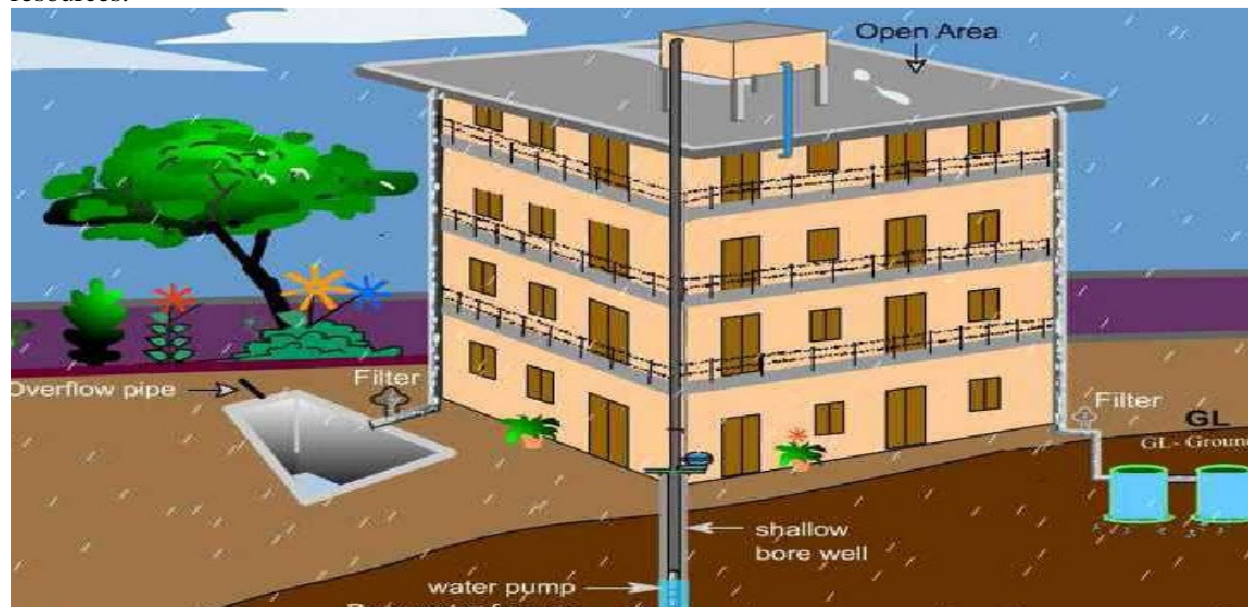
Fig.-3: Roof Top Rain Water Harvesting Source: Images on Internet
