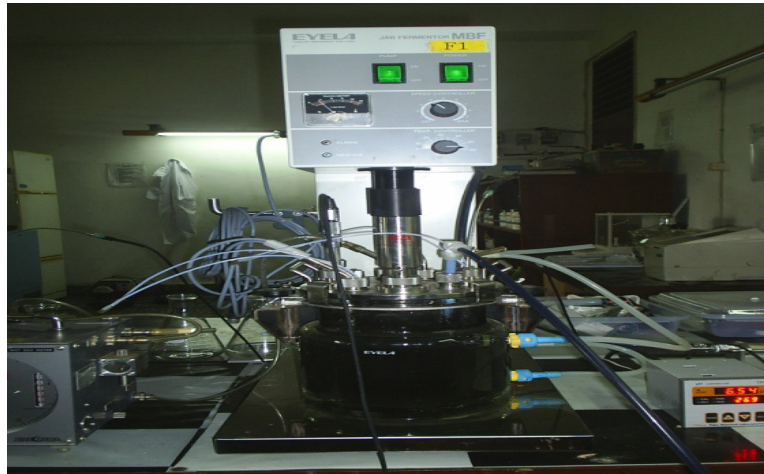
Fig.-1: A two-liter digester used for POME fermentation
