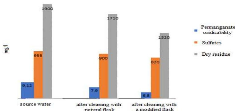
Fig.-4: Results of the Analysis of Underground Water in the Village of Dzhangala after Purification Using the Original and Modified Sorbent
