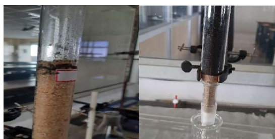
Fig.-2: Experimental Setup for Column Study using Corn Cob
