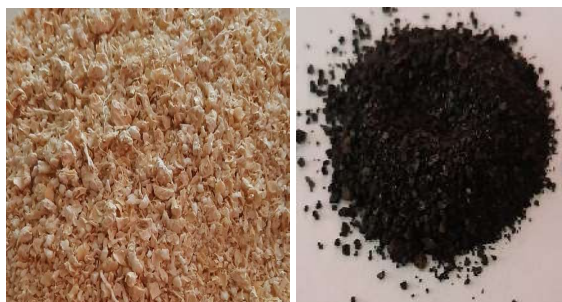
Fig.-1: Corn Cob as (a). Powdered Corn Cob and (b) Biochar
