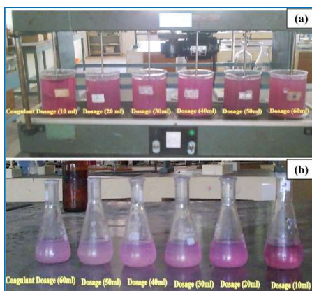
Fig.-2: (a) Jar Test Apparatus, (b) Filtrate Solution from Jar Test
