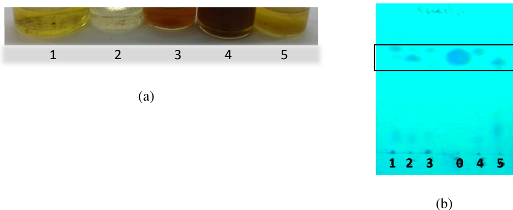
Fig.-7: Identification of Octyl p-methoxycinnamate (OPMC) by transesterification method. (a) The yellow viscous liquid of OPMC. (b) Chromatogram of OPMC standard (0) and OPMC on different time reaction of synthesis using n-hexan:ethyl acetate (7.5:2.5) as eluent under UV 254 nm.
