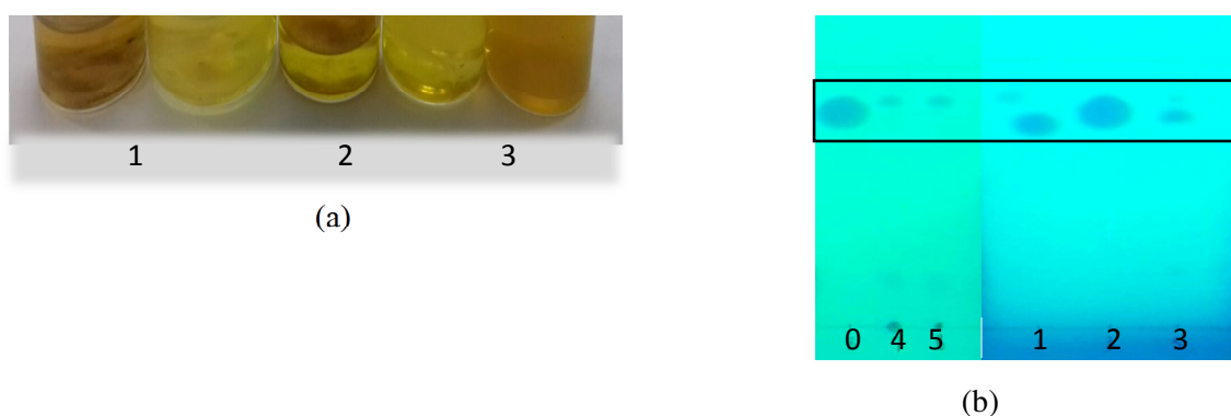
Fig.-5: Identification of Octyl p-methoxycinnamate (OPMC) by esterification method. (a) The yellow viscous liquid of OPMC. (b) Chromatogram of OPMC standard (0) and OPMC on different time reaction of synthesis using n-hexan:ethyl acetate (7.5:2.5) as eluent under UV 254 nm.
