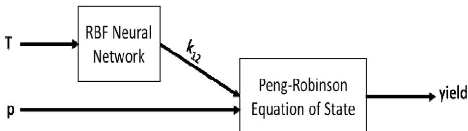
Fig.-3: Proposed Hybrid Model Schematic Diagram<sup>67</sup>.
