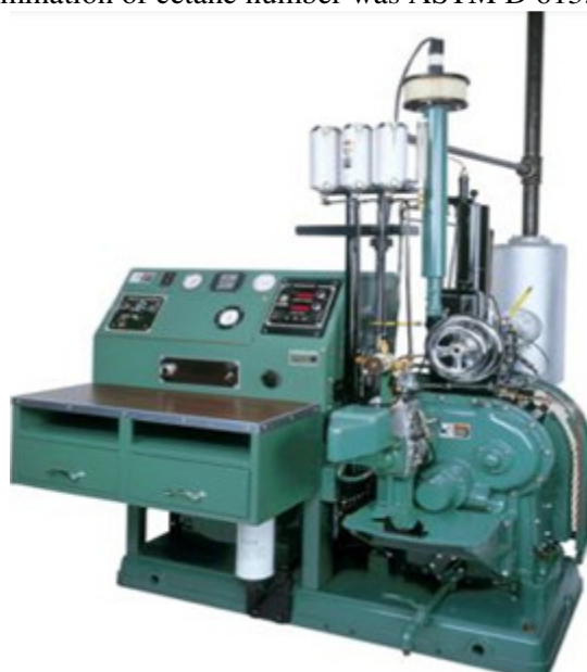
Fig.-2: Image of a Typical CFR Cetane Engine
