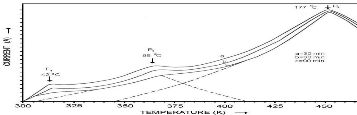
**Fig.-2:** TSC Spectrum of acrylonitrile – isobornylmethacrylate
