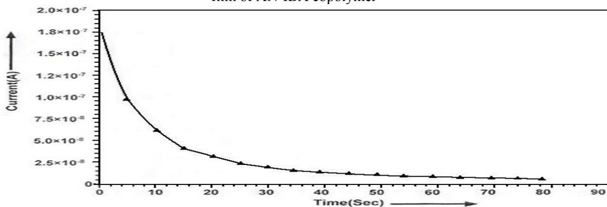
Fig.-7:Decay of current with time for potential applied to an irradiated (Voltage 120V) film of AN-IBA copolymer
