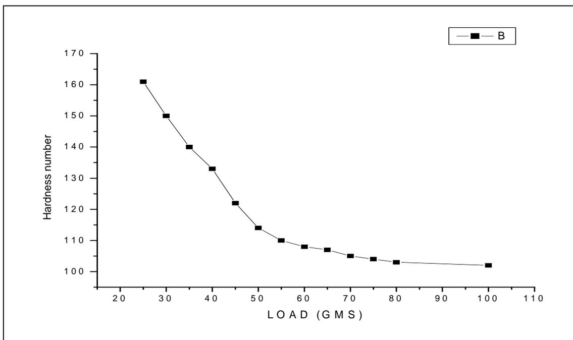
Fig.-4: variation of micro-hardness number with load.
