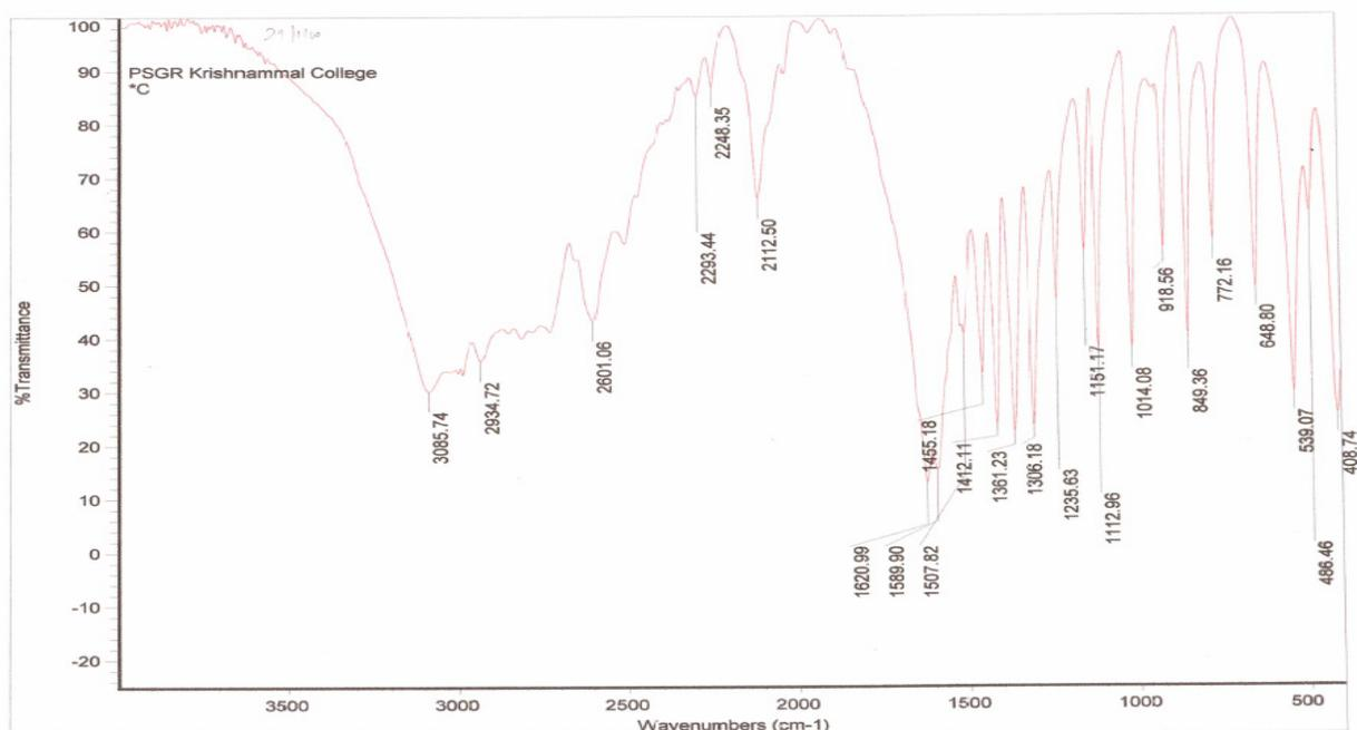
Fig.-1: FTIR Spectrum of Alanine Potassium Chloride (APC)
