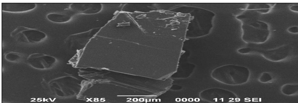
Fig.-4A: SEM Photograph of Alanine Potassium Chloride (APC)
