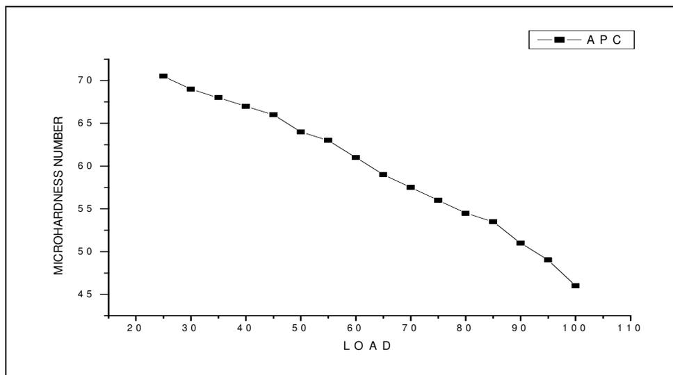
Fig.-5A: Variation of micro Hardness number with load
