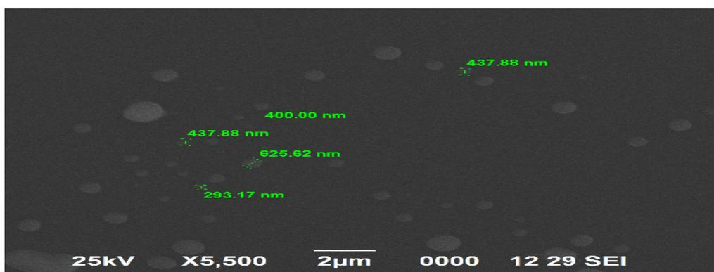
Fig.-4D: SEM Photograph of Alanine Potassium Chloride (APC)
