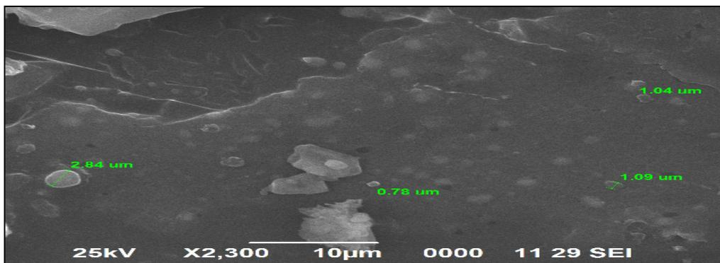
Fig.-4B: SEM Photograph of Alanine Potassium Chloride (APC)
