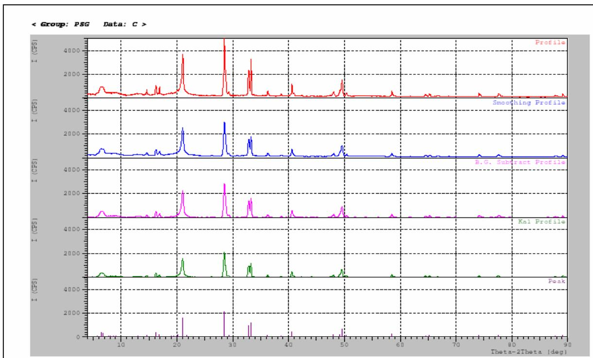
Fig.-2: Powder XRD pattern of Alanine Potassium Chloride (APC)
