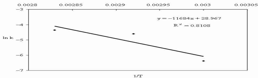
Fig.-3: Determining activation energy.
