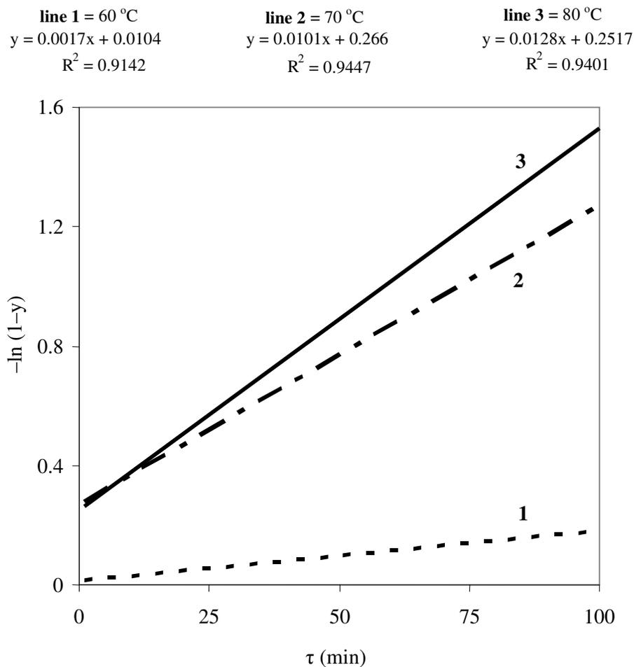
Fig.-2: Rate of enzymatic liquefying of starch to soluble glucose at temperatures of 60, 70 and 80 °C.
