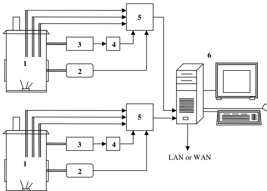
Legend: 1–fermenting tub, 2–heating control unit, 3–flow recorder, 4–analogue-digital convertor, 5–interface, 6–personal computer
