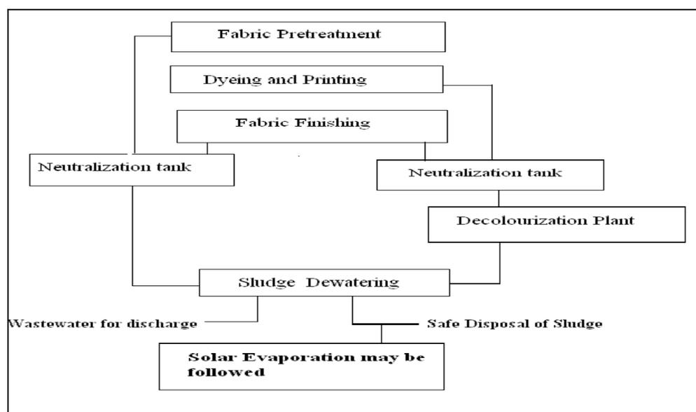
Fig.- 1: Water treatment plant at textile industries
