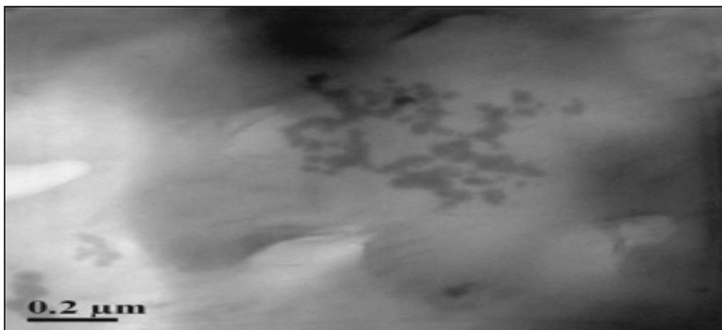
Fig.-11: TEM micrograph of PBT-PET 80-20 with 5 % MMT clay
