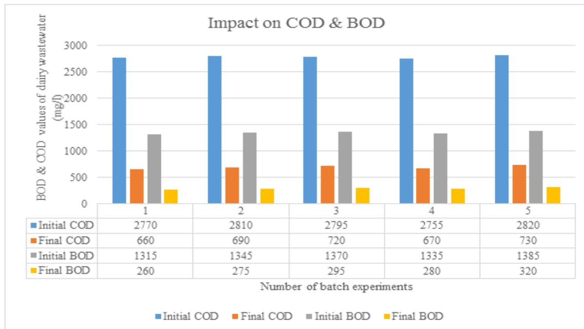
Fig.-3: Impact of MAP and HAP crystallization on COD & BOD values
