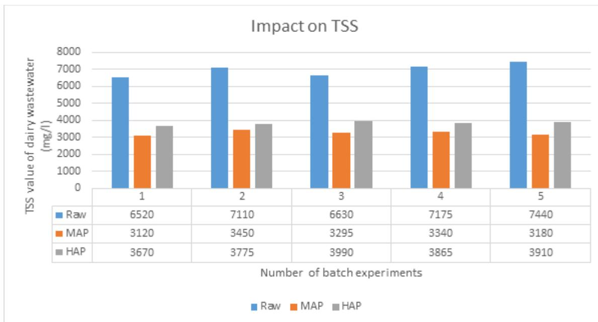
Fig.-4: Impact of MAP and HAP crystallization on the total suspended solids (TSS)
