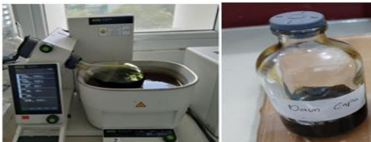
Fig.-6: Evaporation Process for Separating the Solvent from the Capa Leaf Extract
