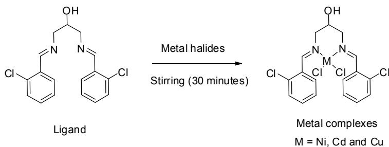
Scheme-1: Preparation of SB Metal Complexes
