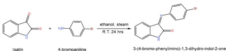
Fig.-1: Synthesis of 3-(4-bromo-phenylimino)-1,3-dihydro-indol-2-one
